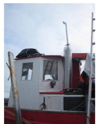
Left: Aage replaces the faulty exhaust pipe on "Agsut". Middle: The defective parts. Right: The new exhaust pipe mounted on "Agsut".
