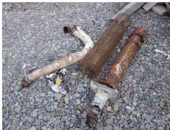
Left: Aage replaces the faulty exhaust pipe on "Agsut". Middle: The defective parts. Right: The new exhaust pipe mounted on "Agsut".
