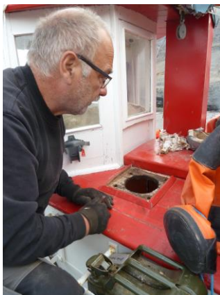
Left: Aage replaces the faulty exhaust pipe on "Agsut". Middle: The defective parts. Right: The new exhaust pipe mounted on "Agsut".
